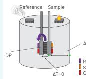
The DP is a measured power differential between the reference and sample cells to maintain a zero temperature between the cells
