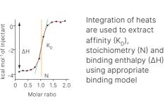
when two molecules interact. Heat is released or absorbed as a result of the redistribution and formation of non-covalent bonds when the interacting molecules go from the free to the bound state.
